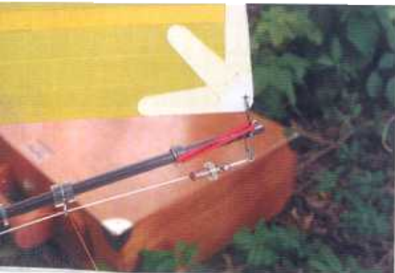
The main outhaul on High Noon has adjustable flow via a third servo
