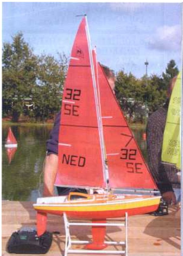
Substantial mast rake on a Dutch boat
