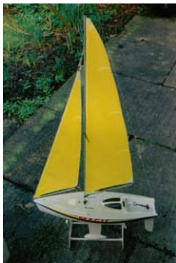
The Mk 1 Micro Magic as supplied, with ali tube mast and spars, rubber grommet sail fittings and yellow colour sails, and scale rudder tiller
