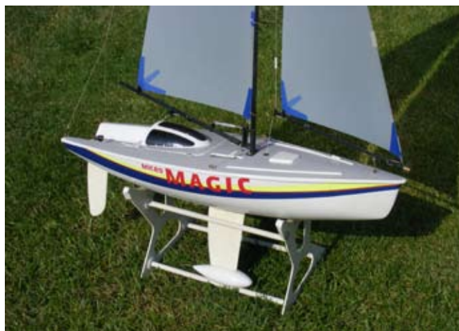
A Mk 1 hull, showing the early profile deck hatch and moulded in false foredeck hatch. The rig has been updated to use carbon spars and Graupner racing fittings
