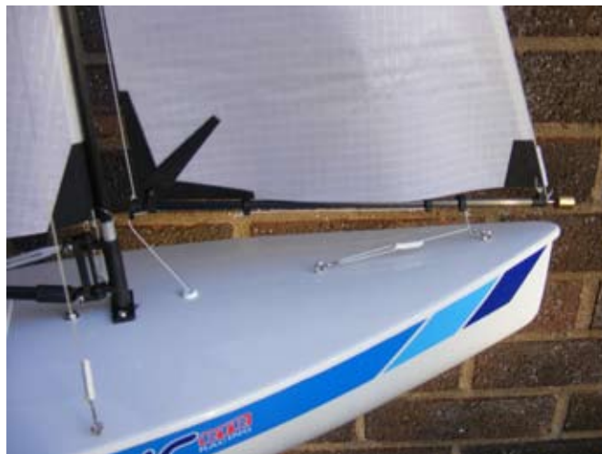
The foresail and boom fittings. The kit instructions assume you are going to leave the rig fitted but a detachable link could be added
