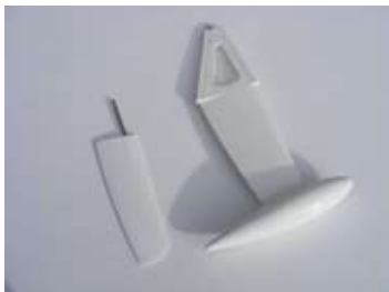
The keel and rudder as supplied. Note the mounded 'spacers' attached to the fin where it enters the hull
