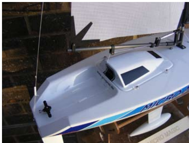
Mainsail boom with gooseneck installed as a compression strut.
