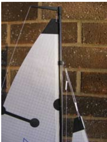
The masthead with moulded plastic backstay and forestay attachments. All supplied with suitable cord ready to go!!
